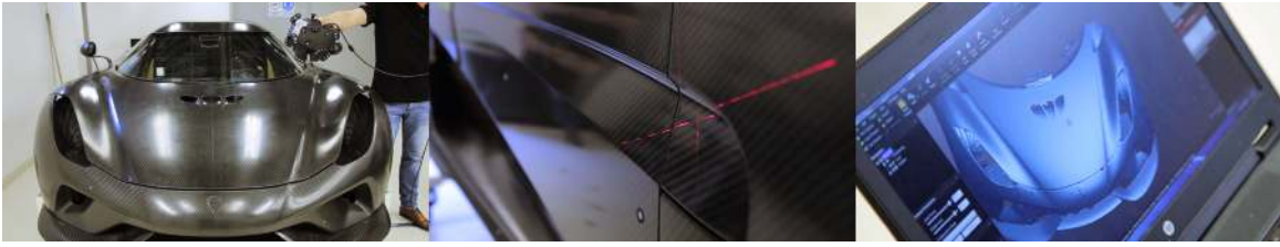
Figure 1.2: Acquisition of a car body using a portable handheld scanner. The scanner uses active stereo and a laser cross to reconstruct the depth. Individual scans are registered via manually-placed markers – white dots on the car body. Image from [Creaform].
